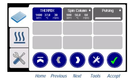
To load the **THERMIX** program, first attach a Heated Module to the unit, then select the **Mixer** page tab, and press the **Home** button, followed by the **Accept** button.
