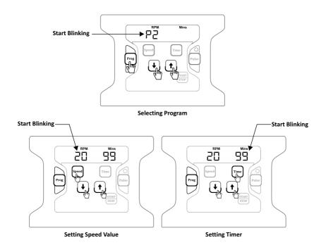
Speed and time value for that particular program is now saved. Press the "Start Button" to start the program mode operation. Once set RPM is reached, the program "Px" (with x = 1 to 9) and its "Speed" & "Time" value will display alternatively.
